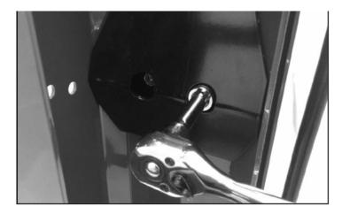
8. If you are not installing a Wheel Chock, skip to step 9. Insert bolts into wheel chock and tighten the locknuts using a 14mm (9/16") socket.
