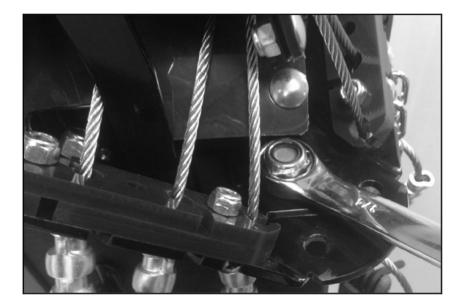
13. Install aluminum casting and then the top cap.
