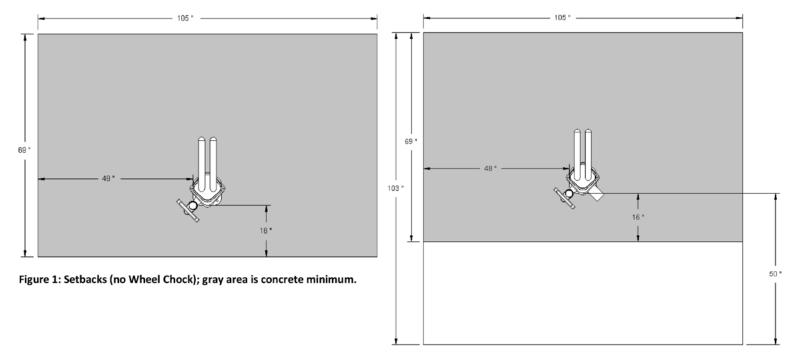
Figure 2: Setbacks (with Wheel Chock); gray area is concrete minimum.
