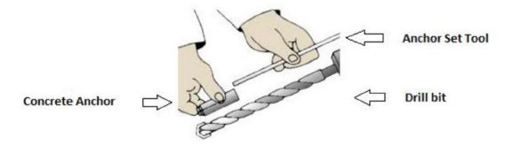
18. Before starting to drill the hole, it is important that eye and ear protection are used. Make sure the hammer drill is in the hammer mode and start drilling your hole.
